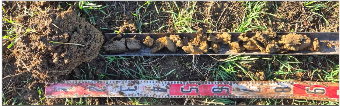
Photo 4: Permeable clay soil (Observation point 8)
